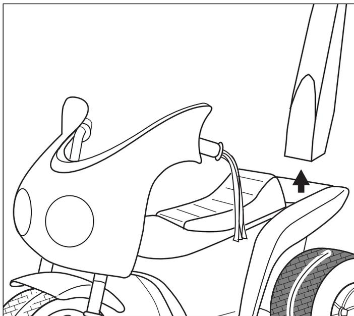
This vehicle features a removable handle so parents can “guide” young drivers. The handle is easy to remove when your child is ready. To remove the handle, use a Phillips screwdriver to loosen and remove the handle retainer screw (#12 x 1/4”) from the back of the vehicle and lift the handle. For storage, insert the screw into the hole in the back side of the handle. Store the handle and screw in a safe place for future use; the handle can be easily re-assembled to the vehicle at any time.
